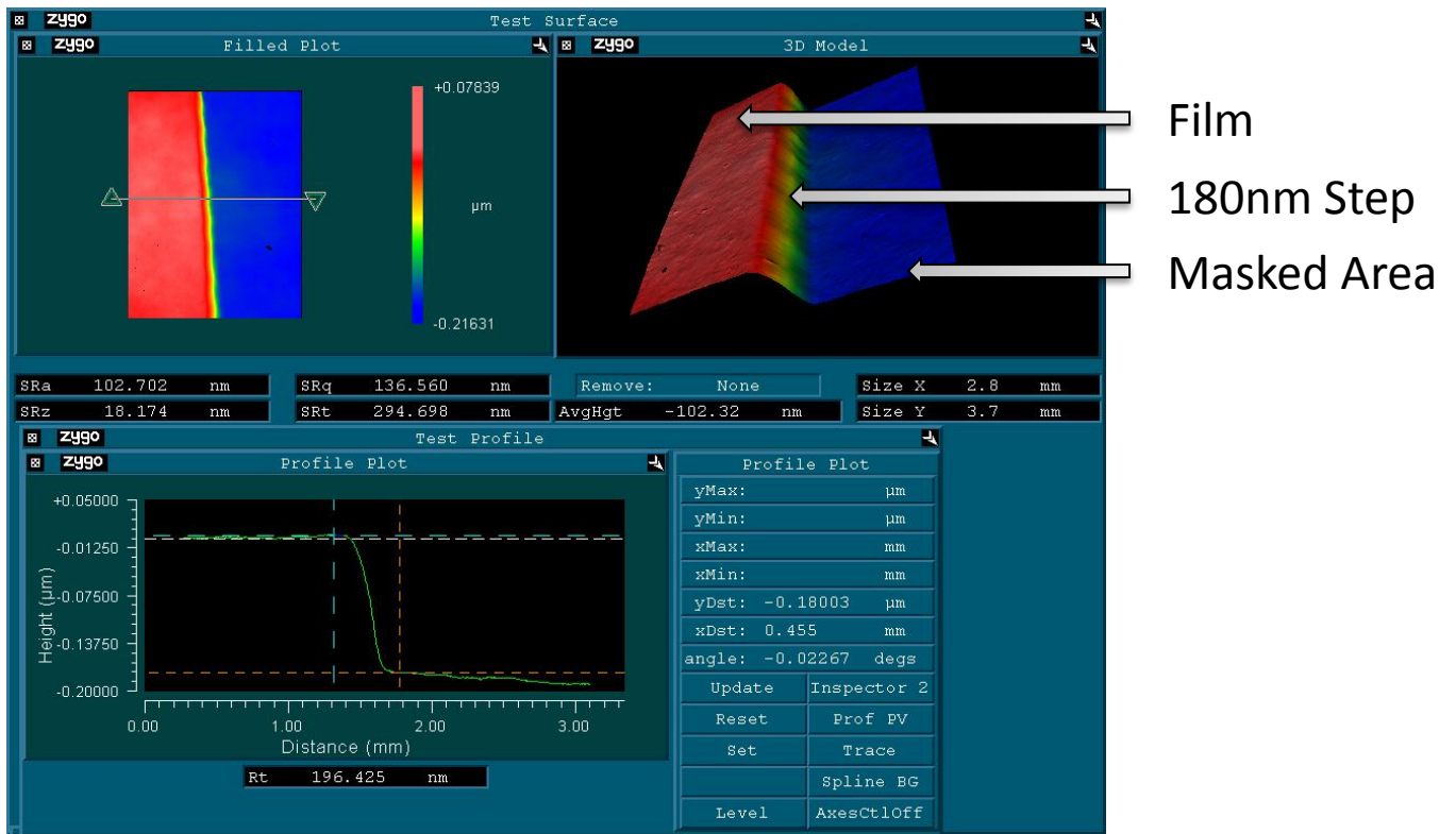
Figure 15 – White light interferometer step height data. The film was found to be 180.0 nm thick with a standard deviation of \pm 2 nm.
